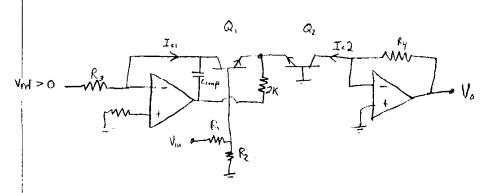
BASIC EXPONENTIAL CONVERTER  $V_0 = \frac{V_{\text{eff}}}{8R_4} e^{\left(\frac{V_{\text{eff}}}{R_1} + R_{\text{eff}} + V_{\text{in}}\right)}$
